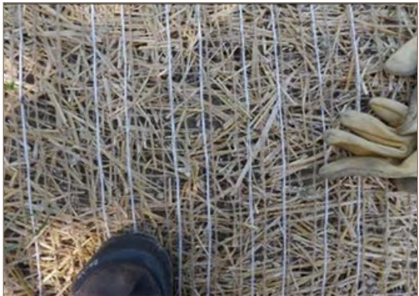
Erosion Control Fabric with a Biodegradable Mesh
