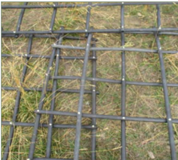
Geo-grid Livestock Deterrent
