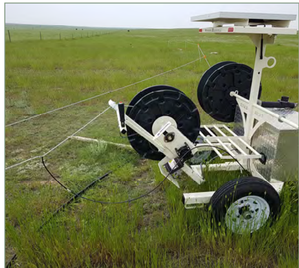
Portable, Solar Powered, Electric Fencing System
